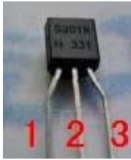
TO-92 package pin arrangement
